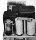
PP-868/U VIBRATOR POWER SUPPLY
