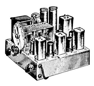
The Browning Laboratories, Winchester, Mass., have announced various component parts for receiving Major Armstrong's wide band frequency modulation method of static-free transmission. Special broadband 3-mc i-f and detection transformers are available as well as a special high-frequency tuner. A completely wired and aligned adapter is in production which may be plugged into the phonograph jack of any receiver.
