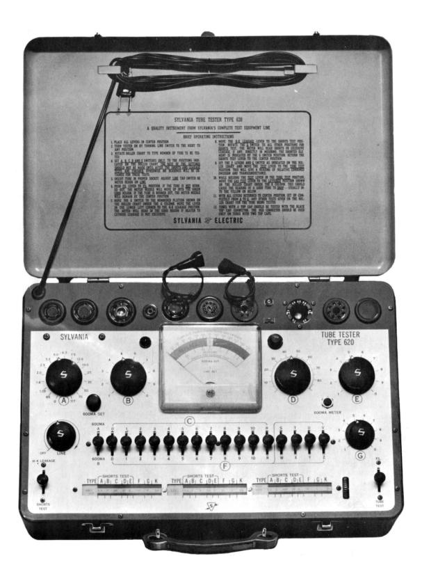
Front Panel of the Type 620 Tube Tester
